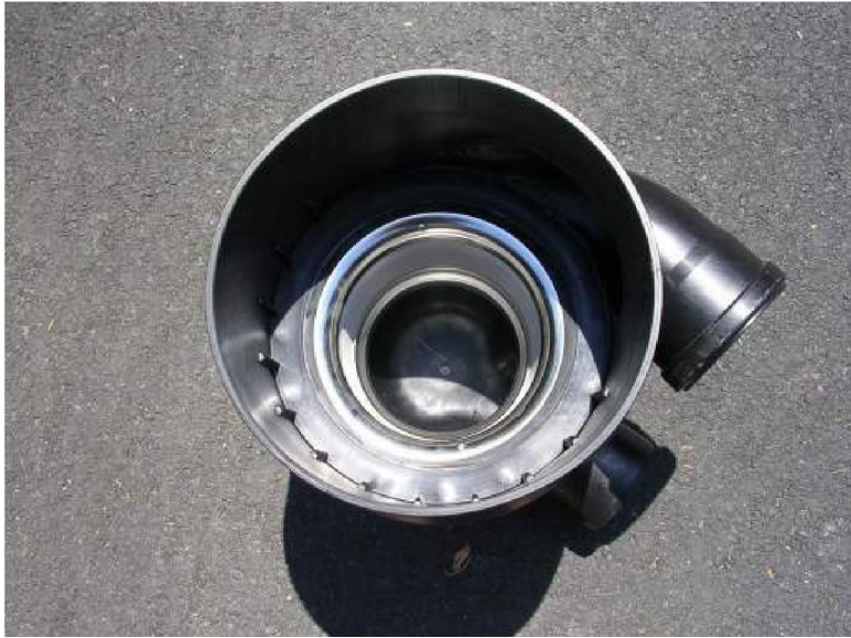
Figure 6.13.12. Interior of Vortex (top) and Installation of Vortex Filter Prior to Backfill (bottom) (Source: VADCR, 2011)
