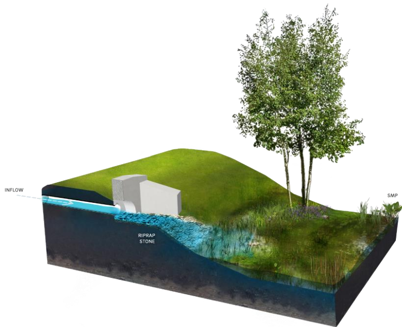
Figure 4-19. Riprap Apron with Typical Features (Source: Fort Wayne, IN Design Standards Manual)
